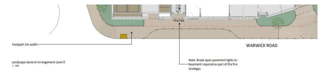
8. The submitted Land Adoption plan (below) which also formed part of the application shows the area of land being given over to the Council for adoption to offset the footway to be used for the pick-up and drop off layby in order that a public pedestrian route of 2 metres could be maintained.
